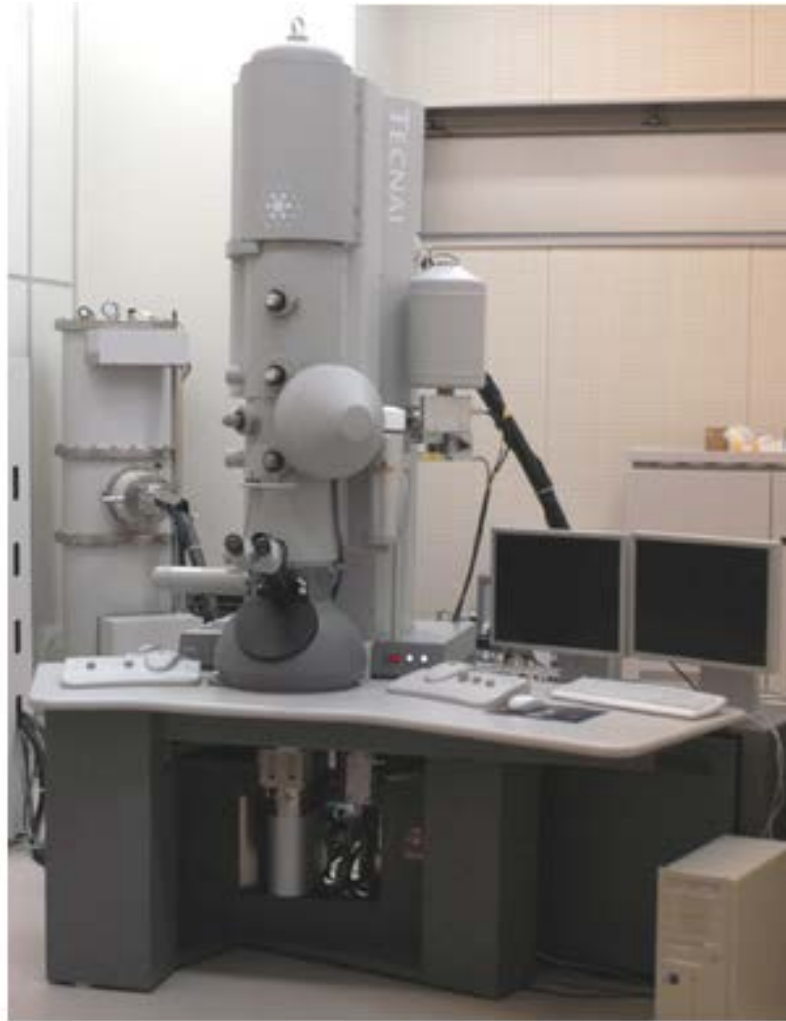
Fig. 2.10 Image of TEM system (FEI Tecnai G 2 F30) [31]
