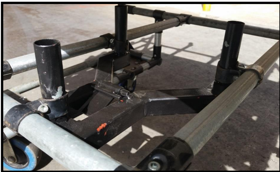
Figure 34. Final Coupling System and Trolley Modifications
