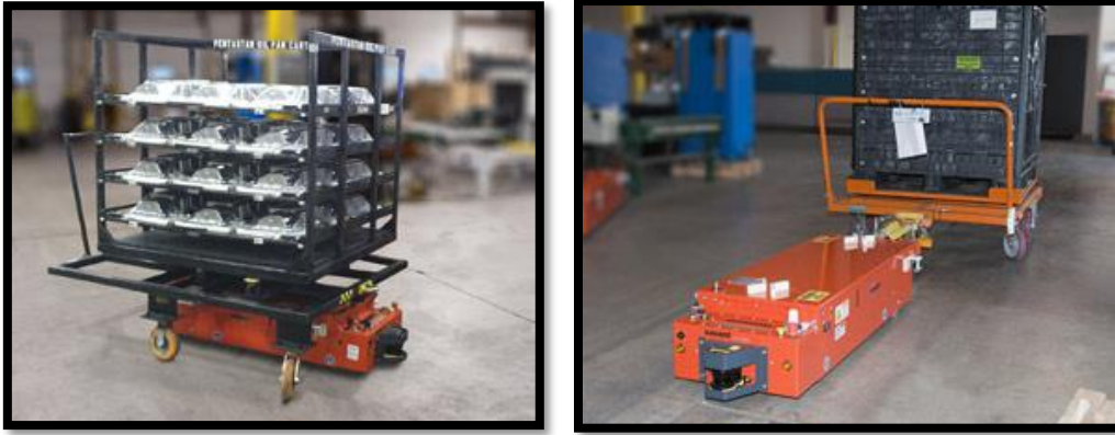
Figure 1. Commercially Available AGV's produced by Savant Automation (2012): AGV Cart Move (Left) and AGV Tow Vehicles (Right)
