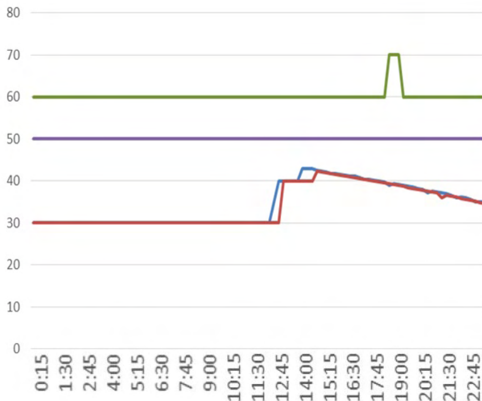
FIGURE 4.5: Simulation results for the second and fourth market model. In the x-axis and y-axis, the simulation time and the clearing price in cents are depicted accordingly. The blue and red lines correspond to the clearing price of C1, C2 respectively. The purple and green lines correspond to the global market clearing price for the second and fourth market case respectively.
