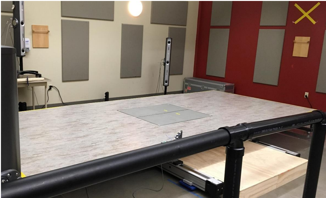
Figure 0-1: Image of assembled translating platform with embedded force platforms and surrounding Optotrak cameras
