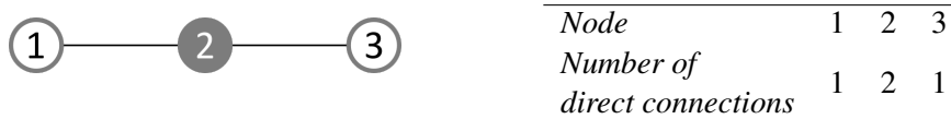
Fig. 4.6 Example 3 of the heuristic used to approximate the position of a node within the network using the information provided by the routing table.
