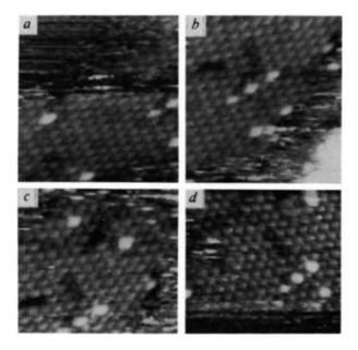
FIG. 1 Sequence of four STM images taken several minutes apart showing ordered arrangements of C<sub>60</sub> clusters on a Au(111) surface. The brighter dots are believed to be due to  $C_{70}$  clusters. Bilinear interpolation has been used in rendering the raw data. The fast scan width (horizontal axis) is ~150 Å and the slow scan width varies owing to piezoelectric creep following translation of the tip to a new area.
