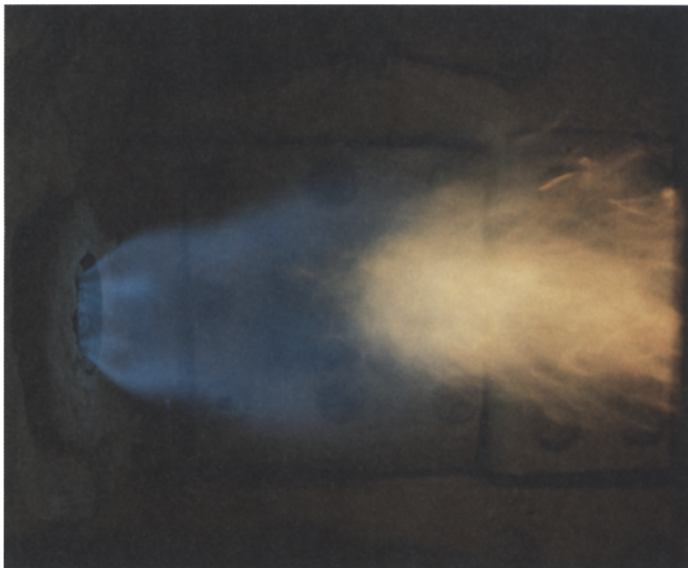
Fig. 2. Photograph of the natural gas flame. The natural gas is burnt with air. The flame has a diameter of approximately 30 cm and a length of 1.5 m. The burner is located in a furnace with optical access via quartz windows. The laser exit window is visible behind the flame
