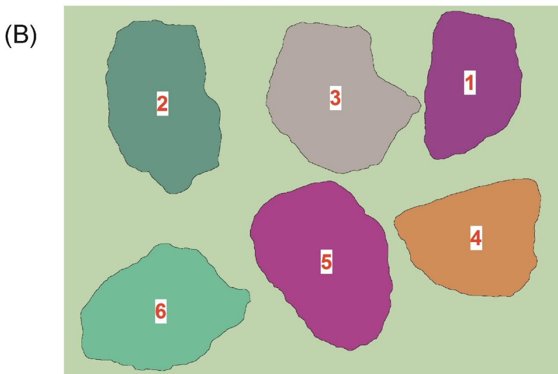
Figure 3.3: Image acquisition of sand grains. (a) Microphotograph of 6 sand grains captured using transmitted light on a microscope. (b) Processed image identifying individual grains to be used for grain shape measurements.
