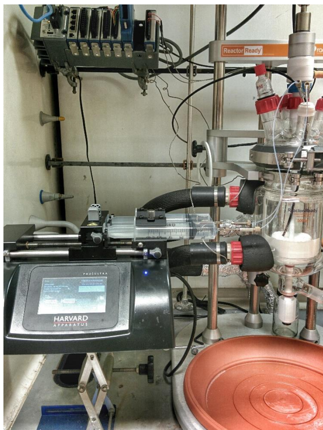
Figure 2.3: Typical set up for the synthesis of macromonomers or multi block copolymers employing a double jacketed reactor and securing a constant monomer addition rate by the use of a syringe pump.
