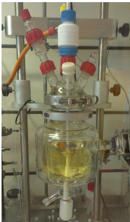
Figure 4.2: The 0.5 L reactor equipped with overhead stirrer, used for the synthesis of the methacrylic macromonomer in large scale.
