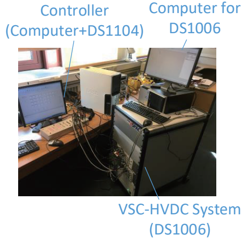
Figure 6: The experiment platform of the HIL test.
