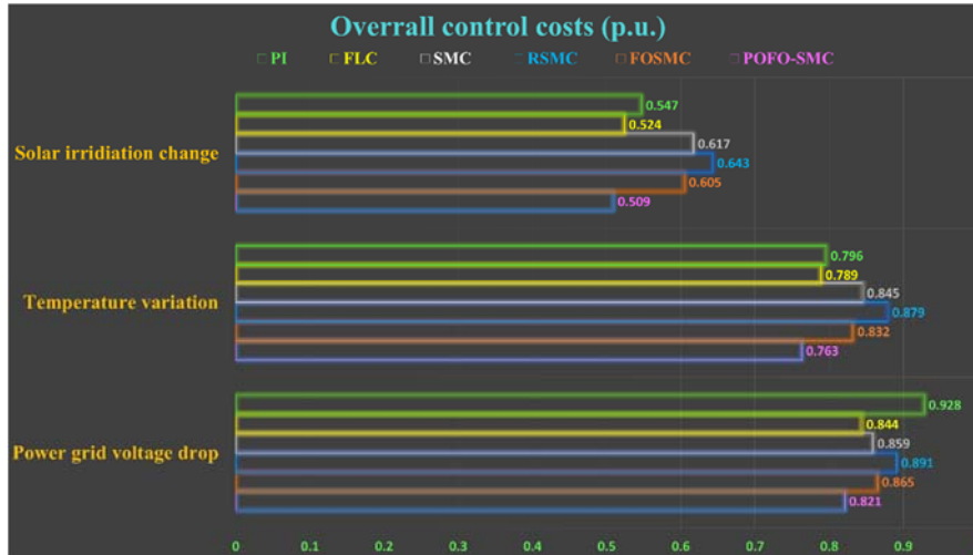
Figure 11. Overall control costs required by different controllers under three cases.
