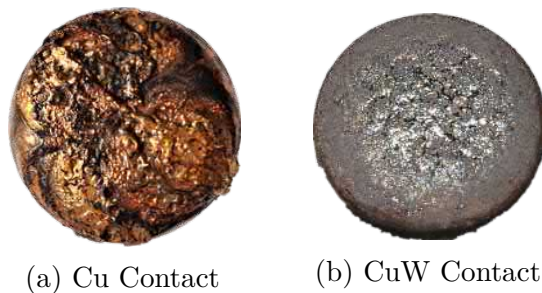
Fig. 1.1 Surface morphology of arcing contacts after current breaking in a HVCB
