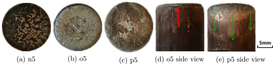
Fig. 3.10 Images of the CuW arcing contact surface subjected to gas blast after current breaking test.
