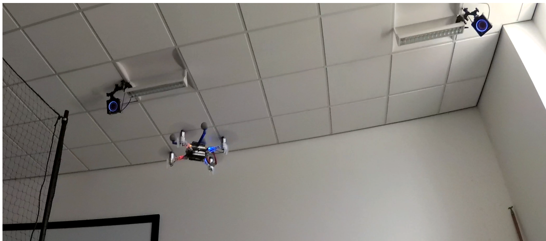
FIGURE 7.13: Employed motion capture system to provide the drones with velocity information and for recording position informations for post-performance evaluation. The tracking cameras can be seen in the top-part of the image.
