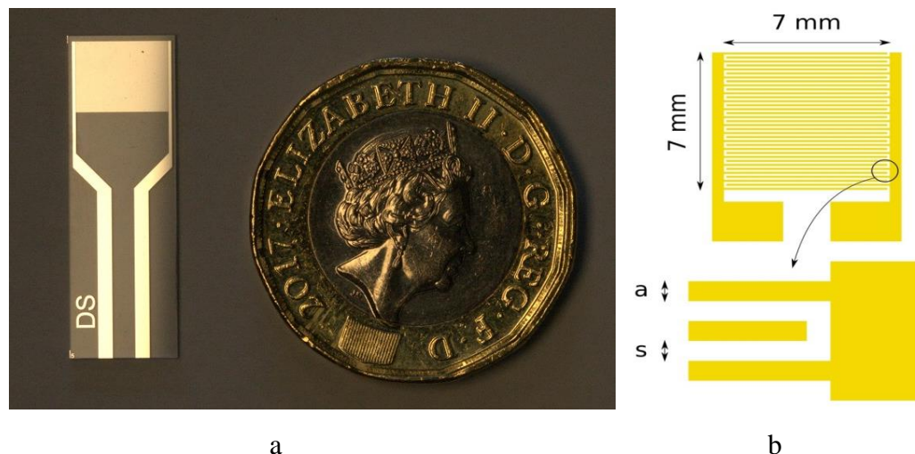
Figure 3-12 a) An image of interdigitated gold electrode (IDEAU5), b) a schematic diagram of IDE
