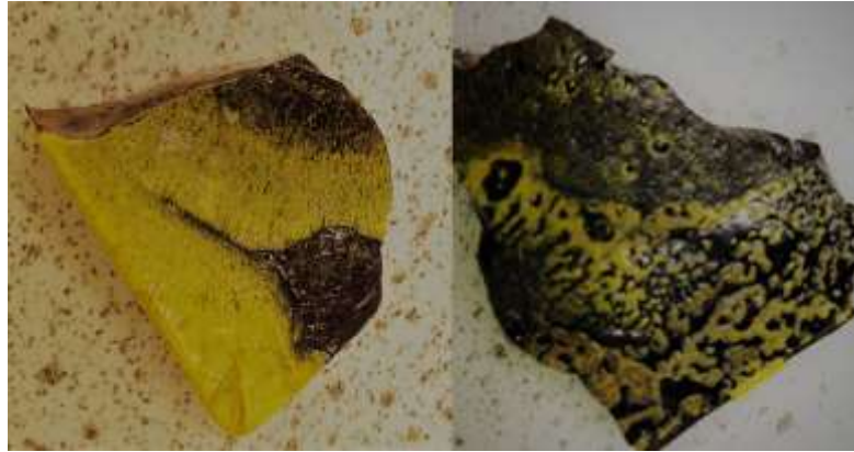
Figure 3.1: “Yellow phase” salt formation in a US LAW simulant glass developed in MERI, Sheffield Hallam University
