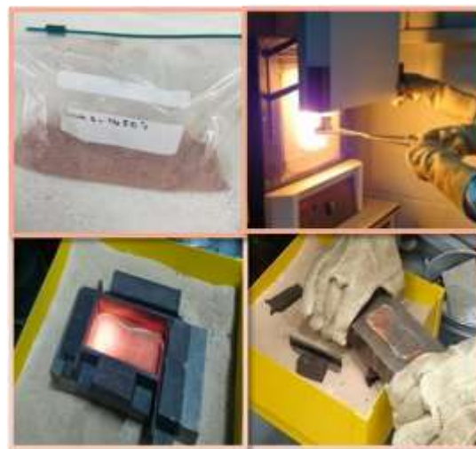
Figure 4.4: Representative photographs of stepwise production of an alkali silicate glass in the MERI lab, Sheffield Hallam University
