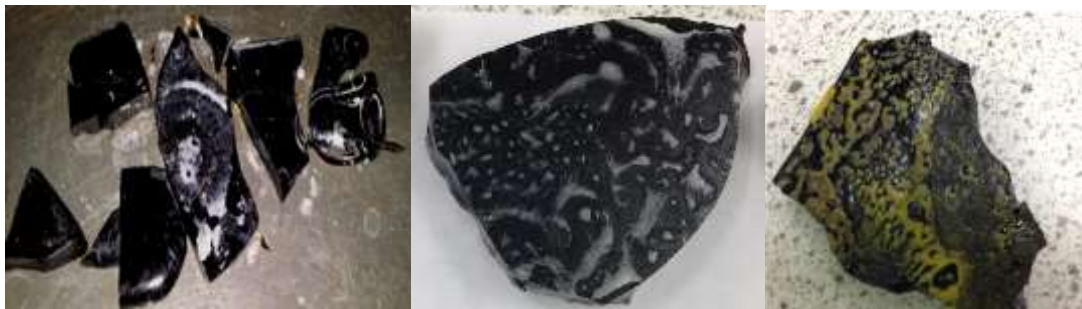
Figure 1.1: Simulated HLW glass (left), LAW glass (middle and right) developed in the MERI lab. A white salt layer on the glass surface appears due to excess sulphate precipitation (left and right), sulphate and chloride (middle). The yellow salt layer (right) is imparted due to presence of chromium in the salt.
