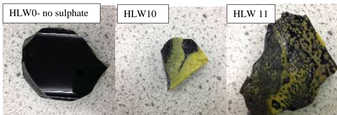
Figure 7.7: DWPF simulated HLW glasses with varying amount of sulphate deposited on the surface.
