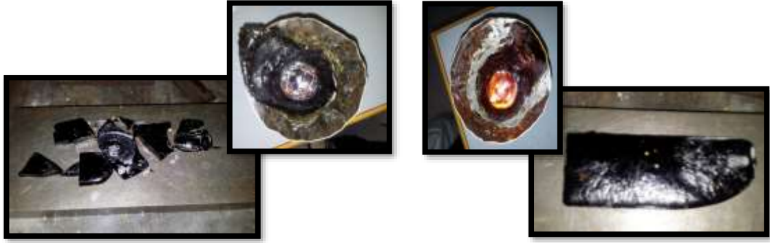
Figure 7.1: Left HLW simulant glass with high SiO 2 shows presence of undissolved sulphate on the surface. Right: Glass with low SiO 2 content shows negligible sulphate flaking on the surface.
