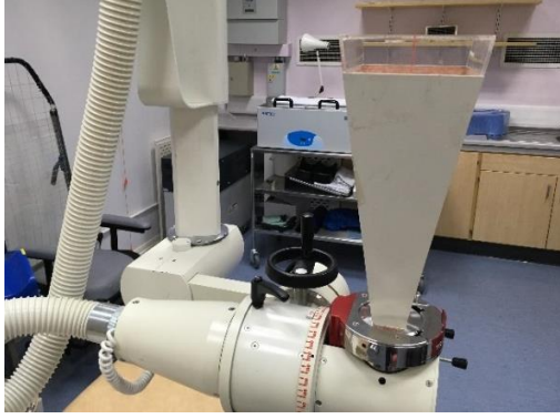
Figure 2.7: Gulmay Xstrahl 200 clinical orthovoltage system.
