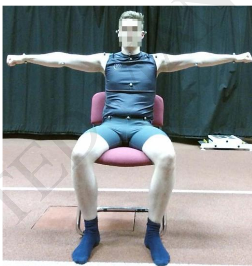
Figure 3: Seated T-Pose posture used as Kinect's ground truth for determining the SD and mean error of joint positions over an exercise.
