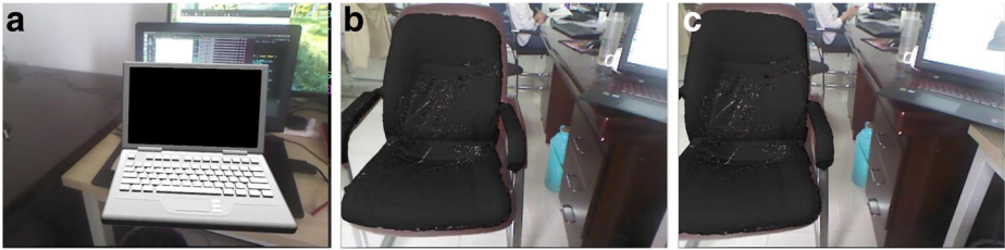
Fig. 6 AR tracking, recognition and registration: a shows the identification and registration of the virtual laptop with a real laptop, b and c show the identification and registration of a 3D model reconstruction from a real chair and registration with a real chair in different view perspectives
