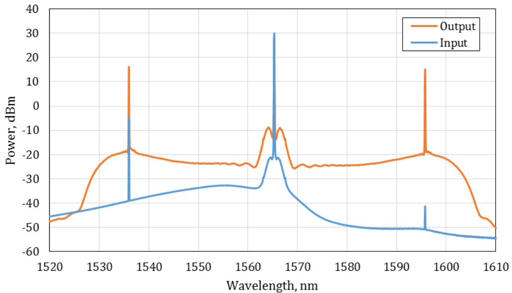
Figure 5.9. Example power spectra at the input and output of FOPA employing a Raman-amplified parametric pump.
