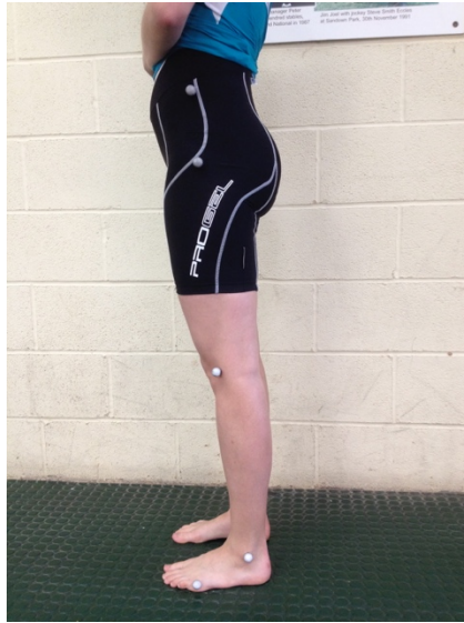
Figure 58. Arrangement of reflective markers. These correspond to the points in figure 54.
