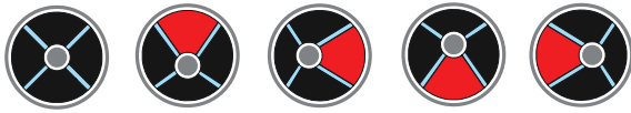
Fig. 2. Actuation principle of the four sector disk DEA. Red shows the actuated segment and consequent movements of the rigid central disk.
