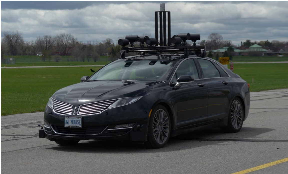
Figure 1.1: The Moose, UW's autonomous vehicle platform, depicted during road testing.
