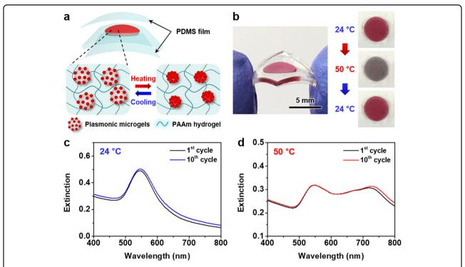
**Fig. 2 Thermoresponsive color shifts of a plasmonic microgel film. a** Schematic illustration of the plasmonic microgel films under the swollen and shrunk states encapsulated between PDMS films. **b** Pictures of the flexible plasmonic microgel films at 24 °C and after heating and cooling for 5 s. UV-Vis spectra for plasmonic microgel films after the first and tenth heating/cooling cycles obtained at **c** 24 °C and **d** 50 °C
