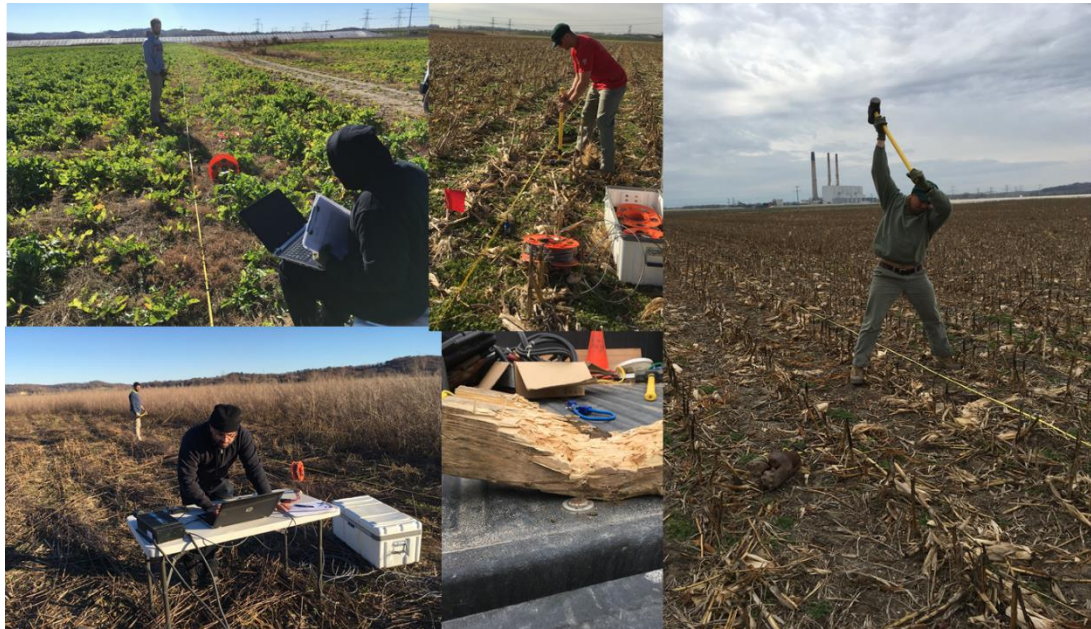
Figure 4.3 – SASW testing at Labadie UWL site, November 2016.
