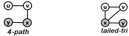
Fig. 2: Example of 4-size non local graphlets. Left: a non-local edge orbit of 4-path, structurally identical to g2 ; right: a non-local edge orbit of tailed-triangle, structurally identical to g5 and g6 .
