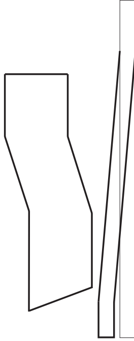
Fig. 7 Deformed state of the inductor and workpiece
