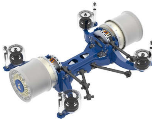
Fig. 3 – The 3D model of DA the 4 th generation with IM-W type ZAwheel SM 530, produced by the firm ZIEHL-ABEGG, Germany
