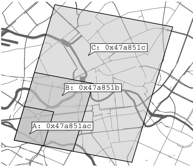
Fig. 2. Hierarchical S2 cell levels. Cell A can be reduced hierarchically to cell B and C. Highlighted is the token representation, that corresponds to Table I, in which the hierarchy can be seen in binary form.
