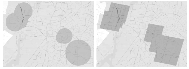
Fig. 4. An example car trace of mobile network position estimates (left), converted to S2 cell encodings (right).
