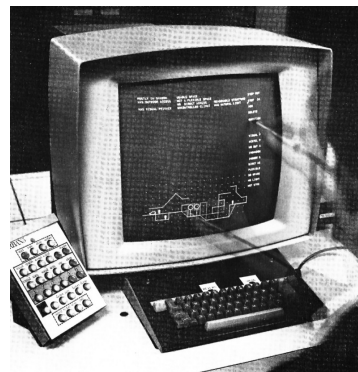
Figure 1. URBAN 5's overlay and the IBM 2250 model 1 cathode-ray-tube used for URBAN 5 (source: openarchitectures.com)
