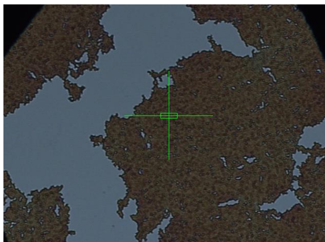
Figure-3.12: Normal image captured by mobile camera (top) and microscopic image (bottom) of the PAN thin films surface spin on to silicon wafer using 50:50 mixture of DMF and MIK as solvent.
