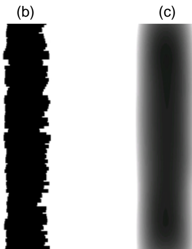
Figure-1.12: (a) The reduction of LER and LWR with RRP time for t-Boc polymer resists with different percentage of protected groups, before (b) and after (c) 300 s of RRP. The roughness of the pattern is significantly decreased by RRP process [9].
