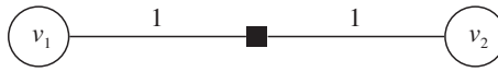
FIGURE 4 Two customers (circles) that need to be served from the depot (rectangle). Assuming that the truck and drone are equally fast, the optimal solution in case no truck-only nodes are allowed has twice the costs of a solution without restrictions
