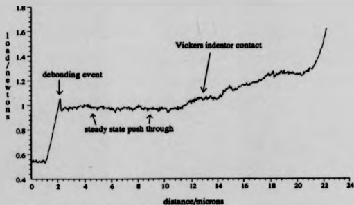
fig.5.31 Load/deflection trace from fibre pushthrough test
