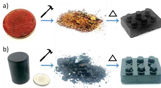
Figure 6. Sulfur polymer samples on, after breaking into powder, centre, and then after being reformed into a monolith again, right: a) sulfur-perillyl alcohol copolymer, and b) sulfur-squalene copolymer. Both samples were made with 50 wt.% sulfur.
