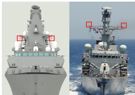
Figure 9: Head-on view of Type 26 (left) and Type 23 (right) showing positions of main anemometers
