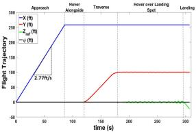
Figure 16: Predictive Tool Input Command for HSDI Task
