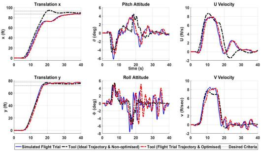
Figure 13: Comparison of Predictive Tool Response and Flight Simulation Trial in PH Task
