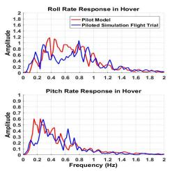
Figure 22: Attitude Rate Response FFT Comparison
