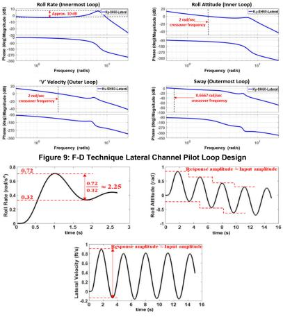
Figure 10: T-D Technique Lateral Channel Pilot Loop Design
