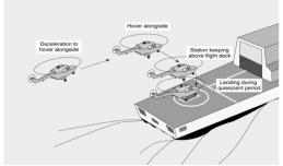
Figure 14: UK RN Standard Deck Landing Approach
