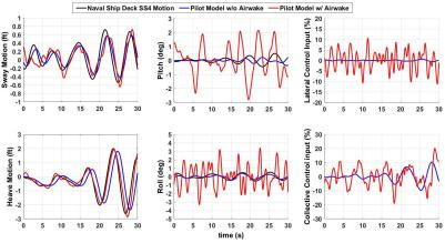
Figure 20: Approximated HSDI Simulation Results using Developed Pilot Model
