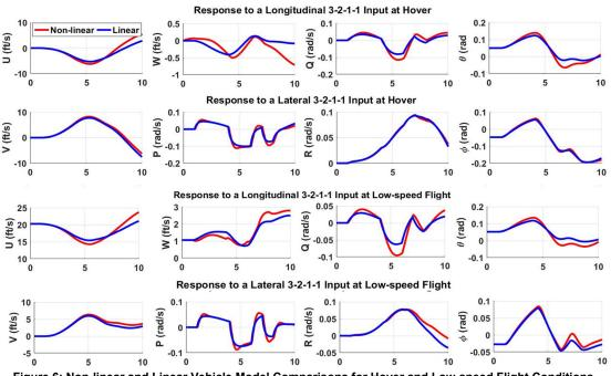
Figure 6: Non-linear and Linear Vehicle Model Comparisons for Hover and Low-speed Flight Conditions
