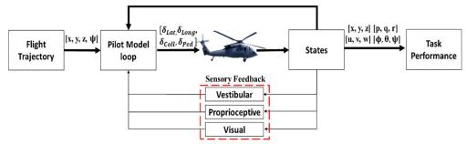
Figure 7: Pilot Model Structure for Motion Sensory Condition
