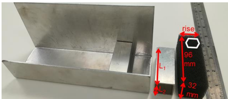
Figure 1: Foam and mold (annotations show cell rise and dimensions. L_1 (x) = 76.5 or 66.5 mm and L_2 (y and z) = 25.5 or 22 mm for VCR = 2 or 3, respectively)
