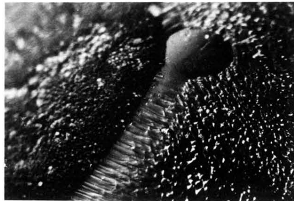
FIG. 1. Growth process on a single-crystal sphere of KDP showing the appearance of a normal crystal face and of a staircase band of faces.
