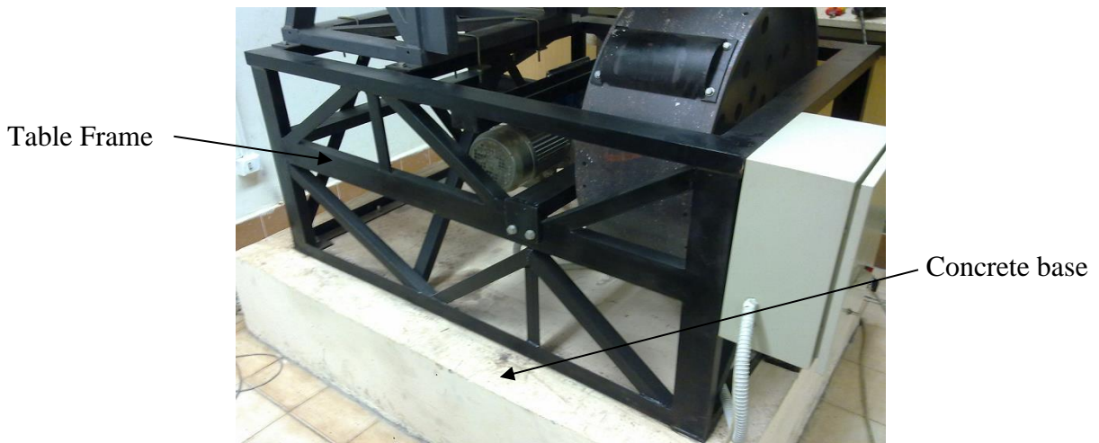
Figure 6.3 Concrete Base and Table Frame
