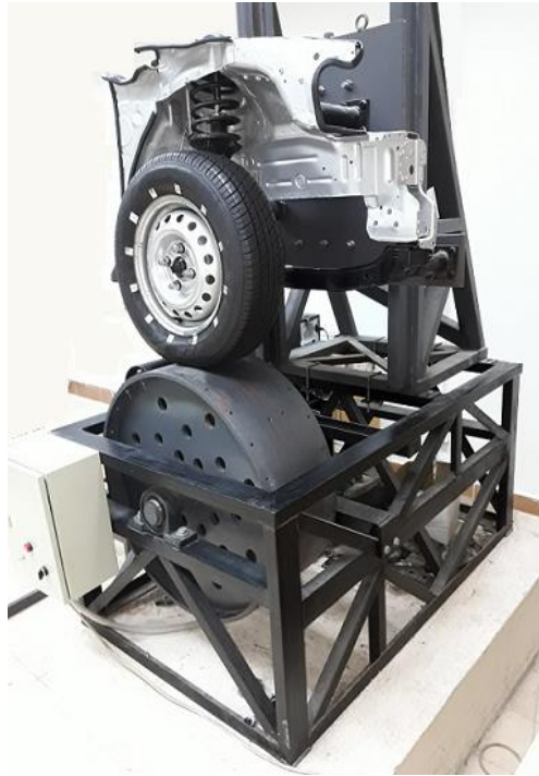
Figure 6.1 Quarter Car Experimental Test Rig
