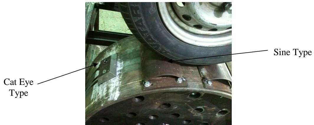
Figure 6.8 Simulation Land Drum with Different Humps
