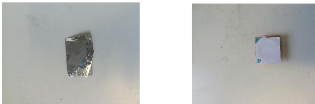
Figure 5.9 – Packaging storage of films in aluminium foils and tablet blister for stability studies at 25 \pm 2 °C and 60 \pm 5 % RH and at 40 \pm 2 °C and 75 \pm 5 % RH.
