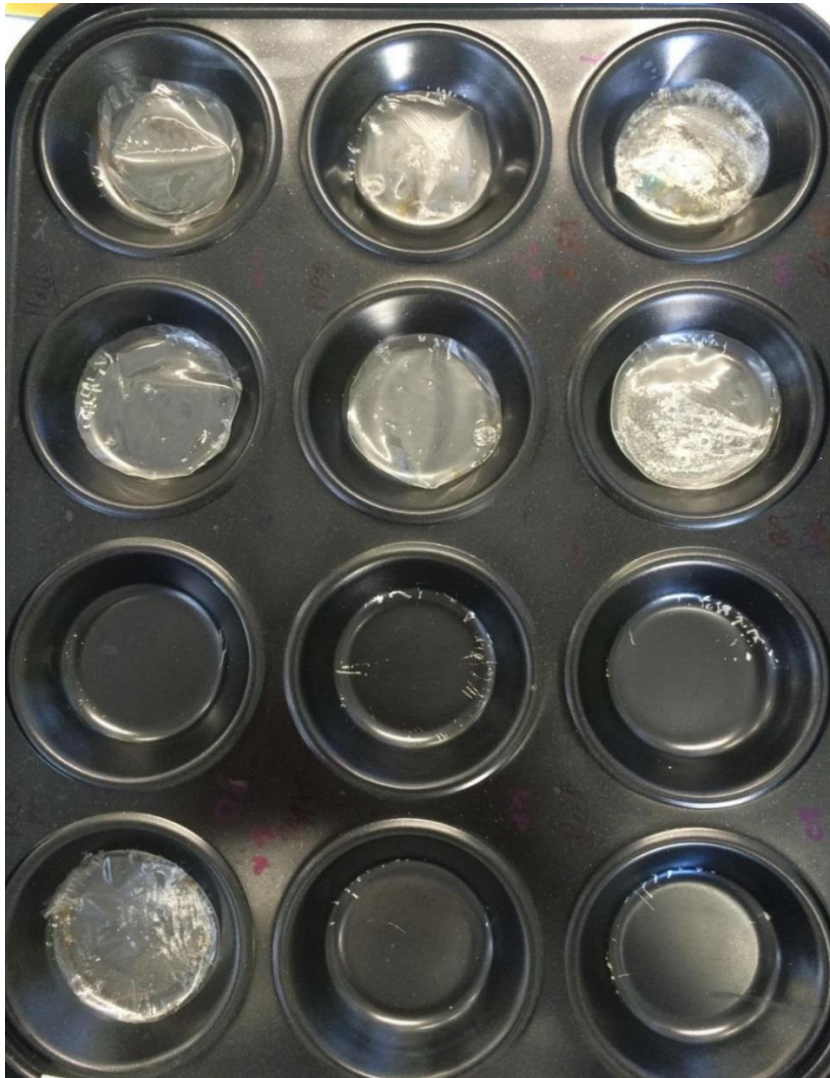
Figure 2.1- Images of ODFs developed by the baking tray method.
