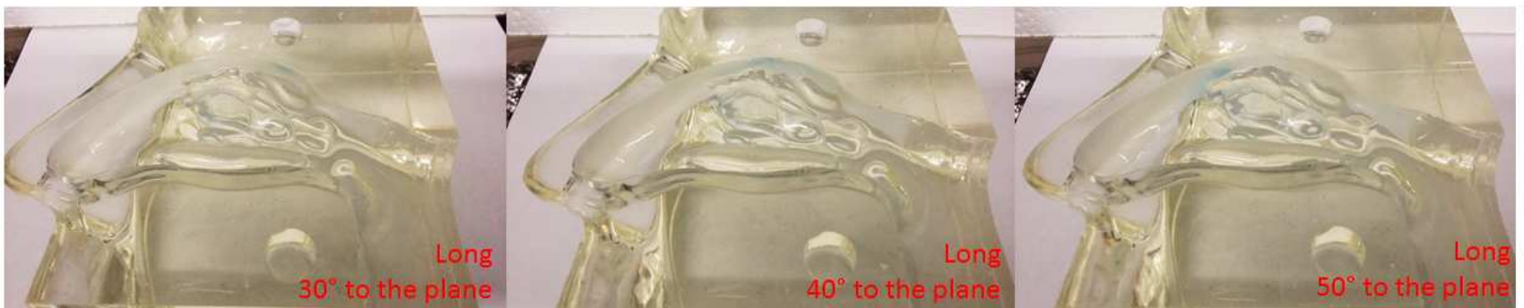
Figure 4-11: Nasal cast deposition of BB pMDI under static air flow and with the 'short' and 'long' nozzle attachments.
