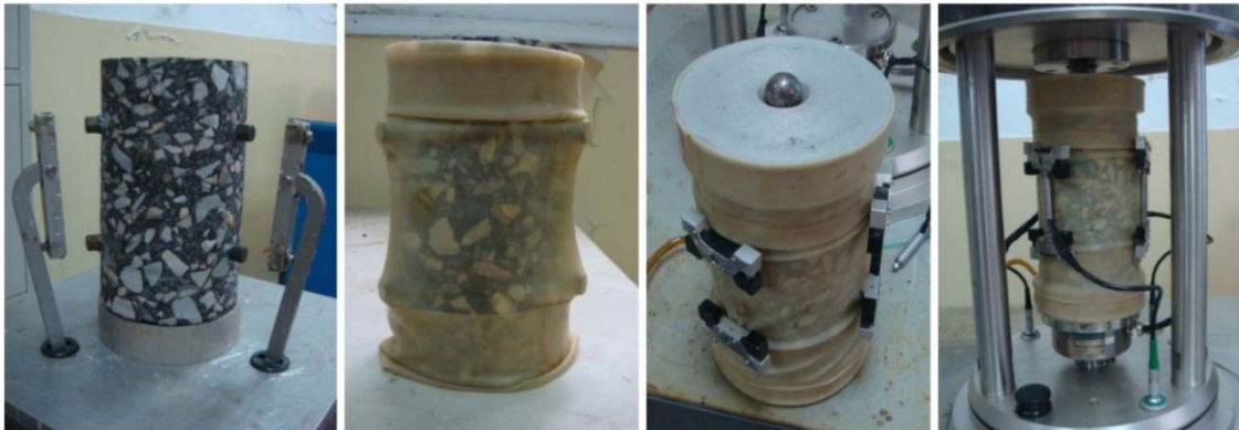
Fig. 3. Details of the experimental setup (Simple Performance Tester)
