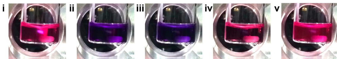
Supplementary Figure 10. Near-infra red light scattering intensity and colour tracking of PDI species during one redox cycle. The system was measured in a semi-batch reactor at 1000 rpm using a 905 nm laser (cf. Supplementary Figure 9) and a camera. PDI (i at t = 0 min, 2.25 mL of a 25 \mu\text{M} solution) is reduced to PDI 2- upon the addition of the reductant (ii, t = 1.2 min) inducing a decrease in the scattering intensity (black curve, left axis) and in the red and blue channel intensity (red and blue curves on the right axis, respectively). Afterwards, PDI 2- was oxidized back to PDI mon (iv, t = 4 min) via PDI - formation (iii, t = 2.75 min), while reaching a minimum in the scattering intensity and a maximum in the blue channel. PDI mon grows via a cooperative polymerization mechanism leading to PDI assem (v, t = 9 min) where an increase of the scattering intensity and the red/blue channel can be observed.
