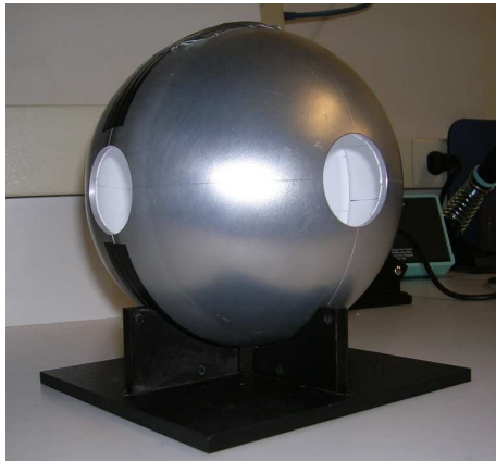
Figure 3. The integrating sphere used in the measurements. The diffusive coating applied to the interior can be seen through two of the ports.
