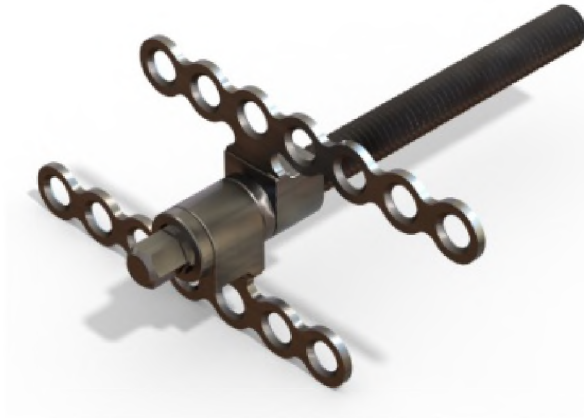
Fig. 2. In the first prototype, the distance between the plates and the distractor was too short, so that it was impossible to adapt them properly to the anterior maxillary wall. The activation head was not long enough and was easily submerged under the mucosa.
