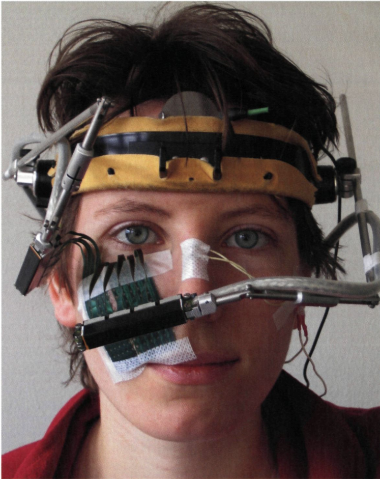
Figure 5-3. Setup for high-density sEMG in the upper facial area. We used two trimmed electrode grids (each consisting of 5 by 12 electrodes) positioned side by side. The cable from the amplifiers was split in two parts behind the head, each containing the connections of one electrode grid. Both cords were guided along two 3-D movable arms that were fixed at the right and left sides of a headset. At the distal end of both arms, two hardprints were mounted serving as a strain relief. The hardprints were equipped with connectors having lockable slots that match with the connection ends of the electrode grids. We secured the borders of the electrode grids in areas that were exposed to moisture or high tensile forces using strips of elastic medical plaster (Fixomull Stretch® Beiersdorf, Hamburg, Germany).
