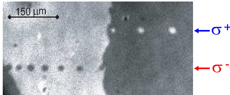
Figure 1.7: The effect of single 40 fs left- and right-handed circularly polarized laser pulses on the magnetic domains in GdFeCo ferrimagnetic metal (from [66, 67]). These experiments showed the possibility of magnetization reversal with a femtosecond stimulus. However, the actual time scales of such a reversal are unclear.
