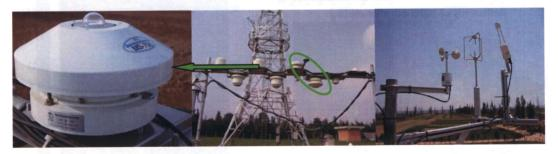
Hyper-spectral radiometer (350nm-1050nm, 10nm res. [max]); Ultrasonic anemometer thermometer; Open path CO2/H2O gas analyzer;
