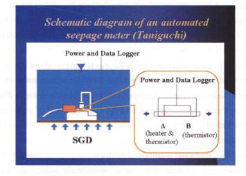
Fig.4 Schematic Diagram of an automated seepage meter
