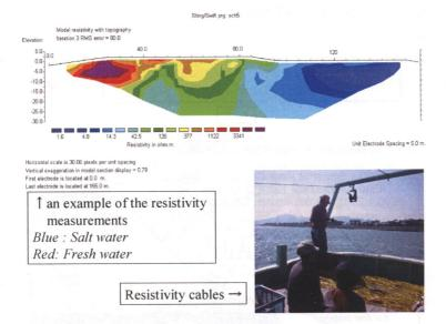
Fig.5 An example of the resistivity measurements
