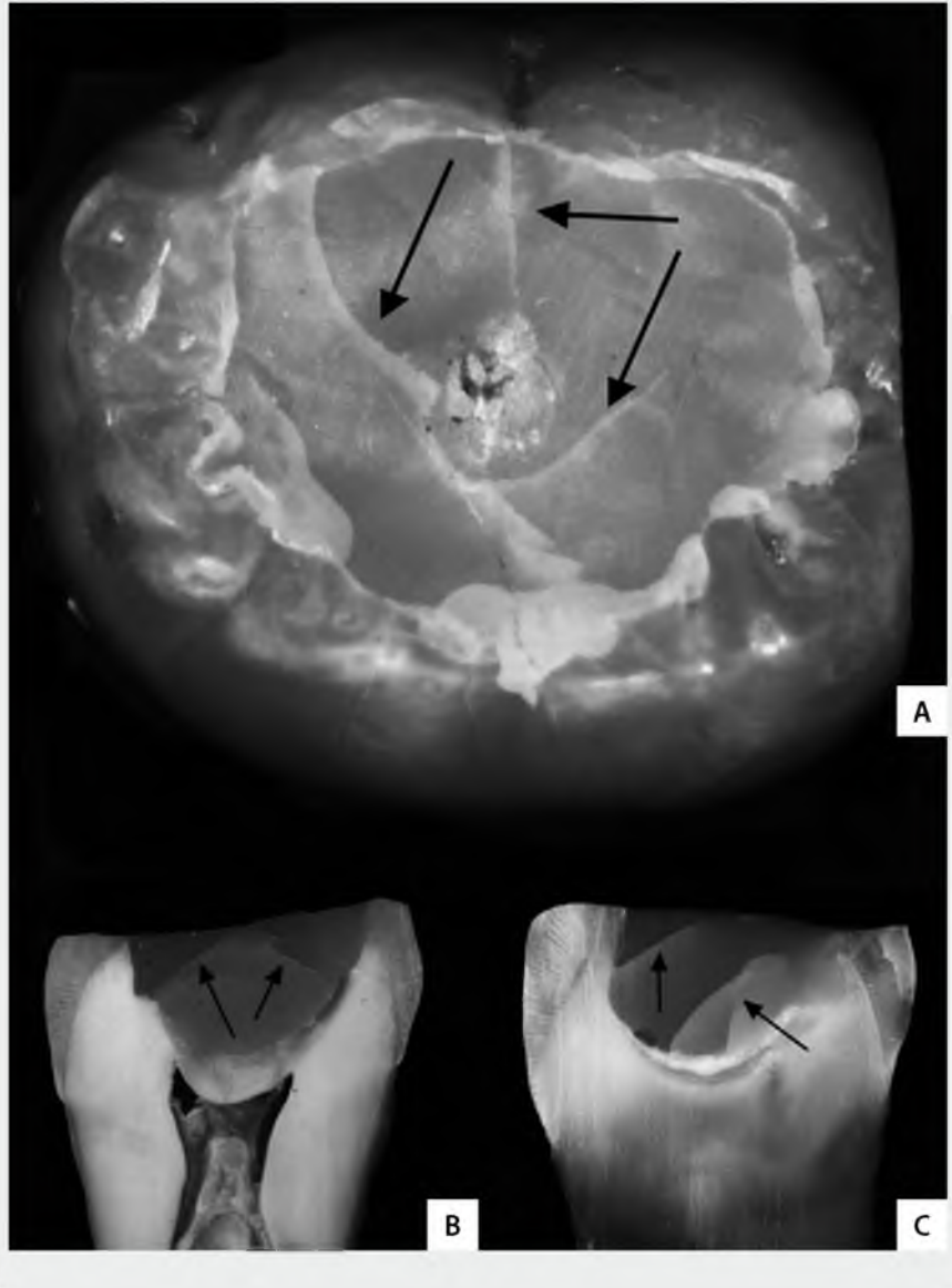
Figure 4 Example of molar from the incomplete excavation group after final failure load test, showing 'ice-cracks' on the occlusal surface (black arrows in A ) and after sectioning the molar (black arrows in B, C ).
