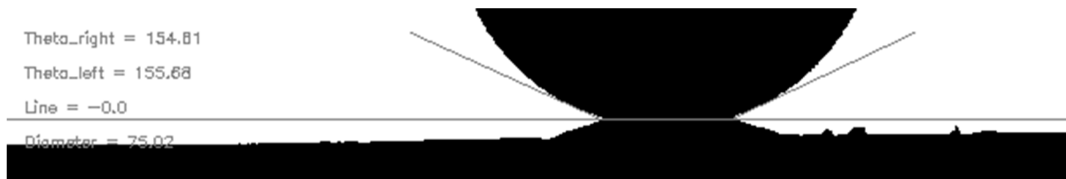
Figure 3.14. Recorded image of the intersection region of a 3 \mu\text{L} droplet on the EWOD electrode. Image analysis with the baseline and the two tangent lines yields the right and the left contact angles as well as the diameter of the contact area.
