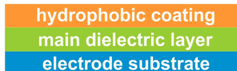
Figure 2.9. General layer structure of EWOD electrodes.
