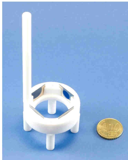
Figure 3.3. PTFE sample holder with four specimens for the cleaning procedures.
